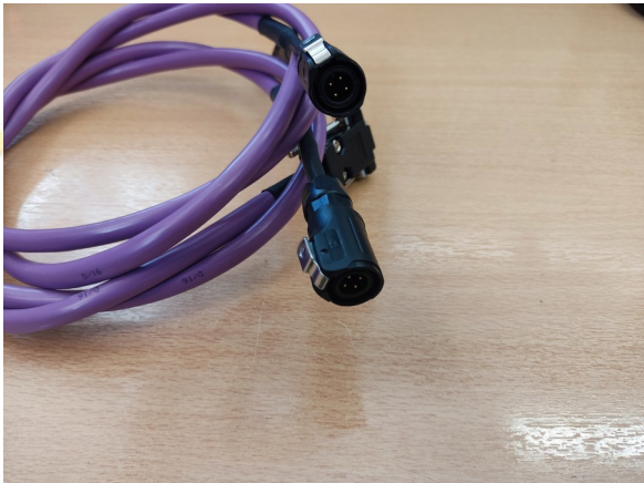
Figure 5: CAN Bus 2 CTC cable (Circular connectors & PC connector via the CAN Bus adaptor).
